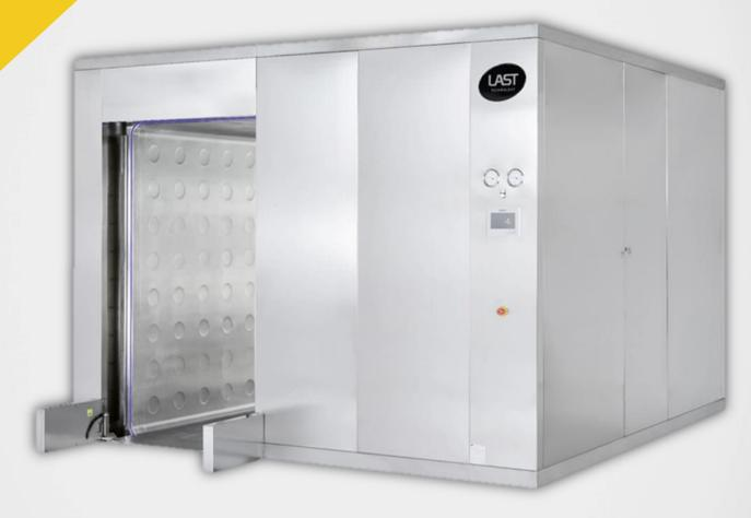
**ETO** processing is widely used today as a low-temperature sterilization method for disposable healthcare devices, medical instruments and pharmaceutical products that cannot withstand conventional high sterilization
