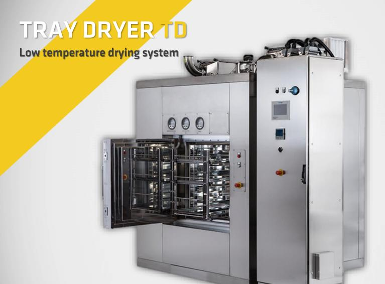
TD is designed for drying solid materials such as powders, fine granulates, machines parts, filters. The machine is provided with an integrated system of CIP or "isolated" filters equipped of "bag-in" and "bag-out" system. ATEX version also available.
