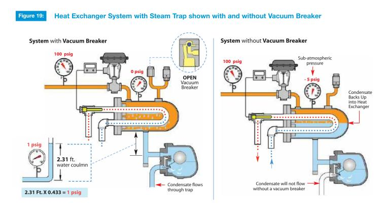
The HX can be properly drained using a steam trap as long as there is no BACK PRESSURE in the condensate return line. If there is back pressure in the condensate return line, a Pumping Trap must be used.
