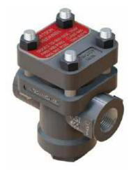
The **Thermodynamic Disc Trap** is simple and compact and an excellent choice for a wide variety of drip applications. They excel in drip applications of pressures ranging from 30 psig to high pressure applications exceeding 3,000 psig, including superheated steam. The ½" TD600L is suitable for most drip applications, and offers reduced size discharge orifice holes which are preferable in terms of performance, longevity, and efficiency.
