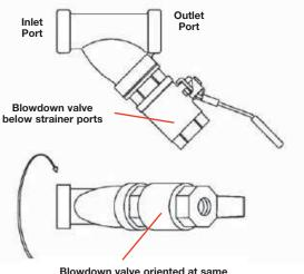
elevation as strainer ports to avoid condensate collection
