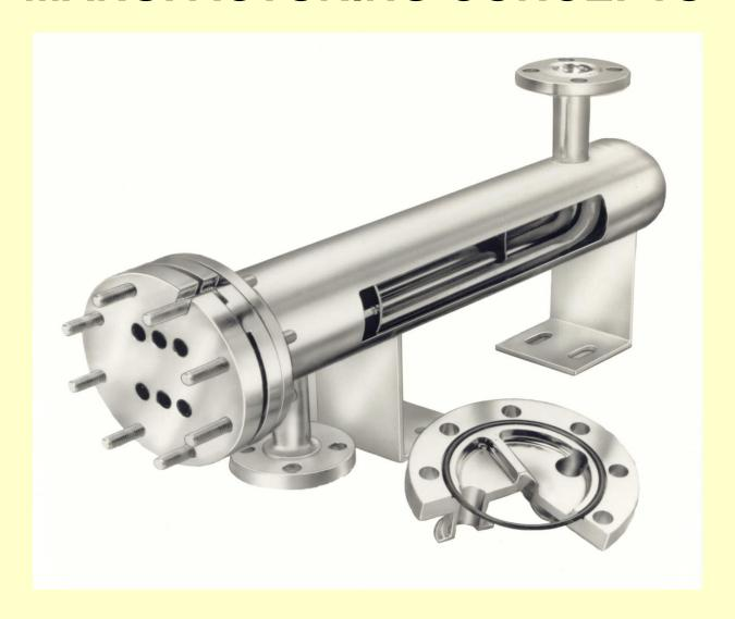
MACHINED O-RING GROOVE AS CLOSE TO THE TRICLAMPS AS POSSIBLE ASSURES NO DEAD LEG FOR BACTERIAL GROWTH AND ALLOWS FOR FULL DRAINABILITY OF TUBESIDE
