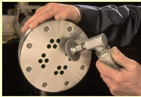
HAND POLISHED TUBESHEET FACES AND TUBE TO TUBESHEET SEAL WELDS, ENSURES NO CREVICES ON PRODUCT SIDE
