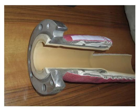
Benefits: Easy to clean: NO Bacteria Proliferation Utmost Safety: Impossible to remove Full flow of the conveyed medium and prevents any contact with metallic part of the fittings
