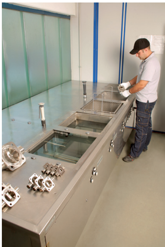
Ultrasonic cleaning of valve bodies
