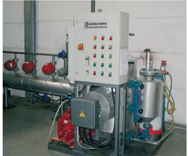
Test stand sterilization process simulation. Cycle and lifetime testing of diaphragms and valves with saturated steam
